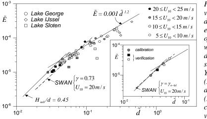
Fig. 4 The observed values of the dimensionless wave energy as a function of the dimensionless water depth for fully developed waves in shallow water of Young and Babanin (2006) and Bottema and Van Vledder (2009). Inset shows calibration and verification results.
