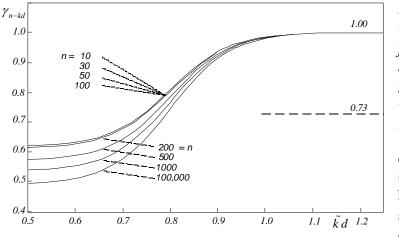
Fig. 1 The calibrated value of  $\gamma_{n-kd}$  as a function of bottom slope n and normalized depth kd, with  $\gamma = 0.73$  as reference.
